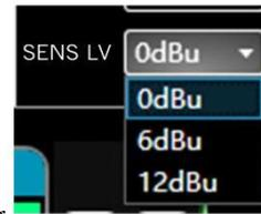
⑤Support 0dBu, 6dBu, 12dBu three-level sensitivity switching
