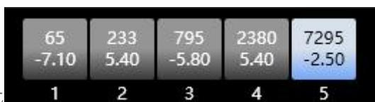
As pic 6.1, below the curve chart, Display all EQ controls and their detailed values, which can be used to locate the position of the controls. Combined with the EQ parameter adjustment items below, the parameter values of each EQ can be accurately adjusted.
